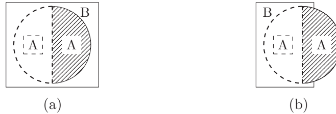
Figure 3.2: Two Examples of Mutual Obscuration. (a) A's projection completely contained in B's projection, (b) A's projection partially overlaps B's projection.
